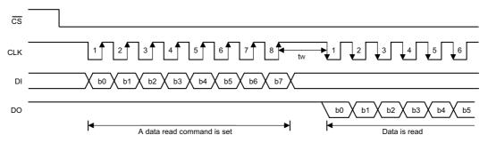
DO must be sure to connect an external pull-high resistor to this pin (1k $\Omega$  to 10k $\Omega$ ). Note: When data is read, a wait time "tw" of 1 $\mu$ s is necessary.
