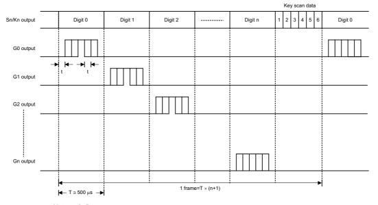
Note: n=0~5 t=1/16T T: pulse width of segment signal is decided by oscillator frequency One cycle of key scanning consists of one frame.
