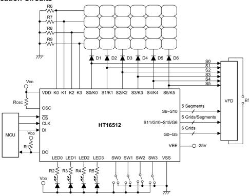
Note:  $R_{OSC} \!\!=\!\! 51 k\Omega$  for oscillator resistor
