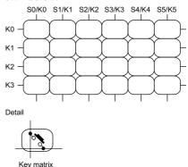
The data of each key is stored as illustrated below, and is read with the read command, starting from the least significant bit.
