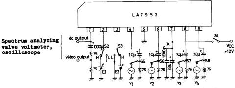
$\ensuremath{^{*}}$  Connect the capacitor for  $V_{CC}$  as close to pin 7 as possible.
