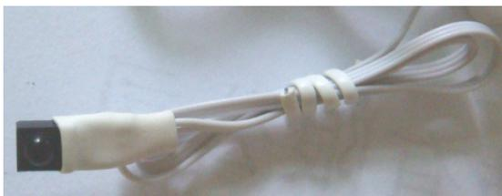
Adopt oblate three-way wire, and connect an infrared receiver to receive an external infrared.
