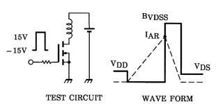
$$\begin{aligned} &R_G = 25~\Omega \\ &V_{DD} = 90~V,~L = 15~mH \end{aligned} \qquad EAS = \frac{1}{2} \cdot L \cdot I^2 \cdot \left(\frac{BVDSS}{BVDSS - VDD}\right) \end{aligned}$$
