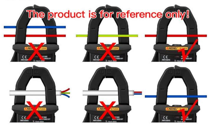
Ac current measurement, can only measure the zero line or fire line, and only a core line, the common electrical appliances in the home power supply line is not measured, because it contains a number of core wire.
