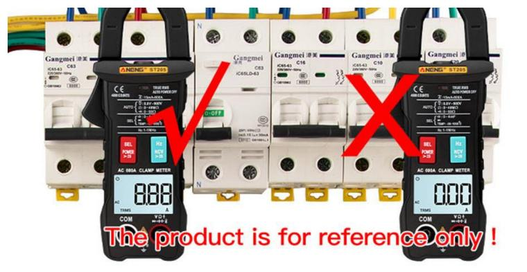
Before measurement, the measured current should be estimated and the appropriate range should be selected. When the current is not known, the maximum range should be selected and the range should be reduced appropriately according to the value. However, the range cannot be converted during measurement.
