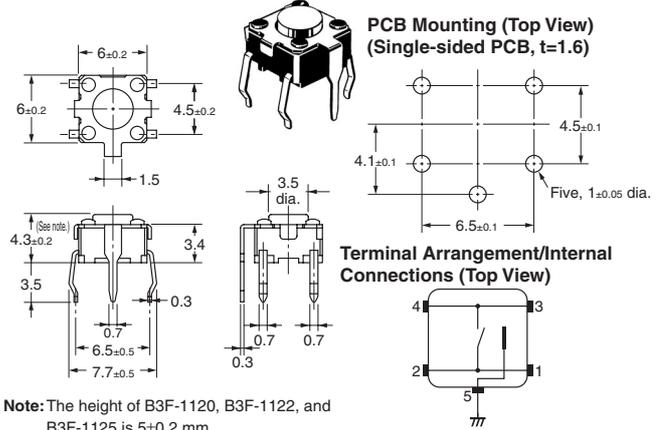
**Note:** The height of B3F-1120, B3F-1122, and B3F-1125 is  $5 \pm 0.2$  mm.
