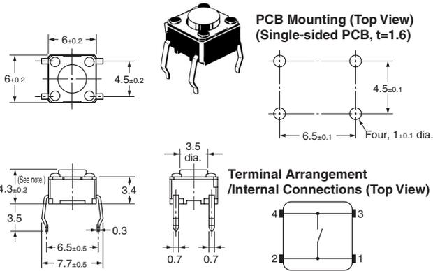
**Note:** The height of B3F-1020, B3F-1022, B3F-1025, and B3F-1026 is  $5 \pm 0.2$  mm.
