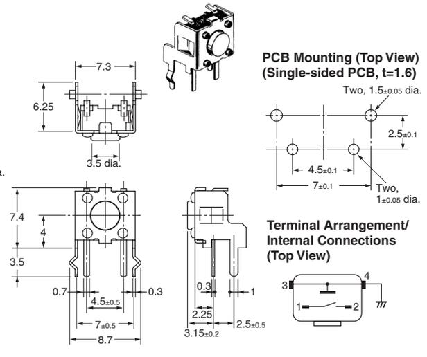
**Side-operated, Flat Plunger Type (Height: 3.85 mm)**
