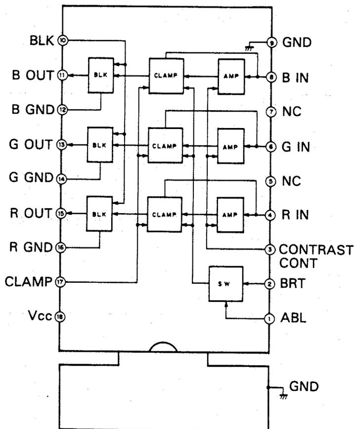
Pin Description and Equivalent Circuit
