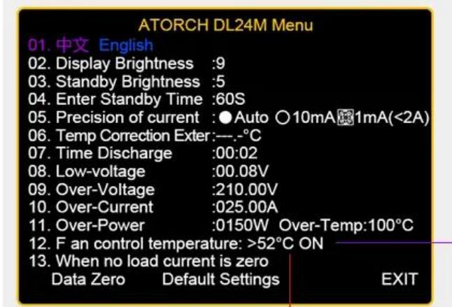
If you set the starting temperature of the fan to 52 ° C, when the fan temperature reaches 52 ° C, the fan will start working, and when the temperature reaches (52 ° C-10 ° C=42 ° C), the fan will stop!
