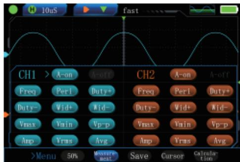
**Save:** Click Save to save the oscilloscope's measurement page in the Screenshot file folder in the machine's USB flash drive as a BMP format image. The image name will be displayed when saving.
