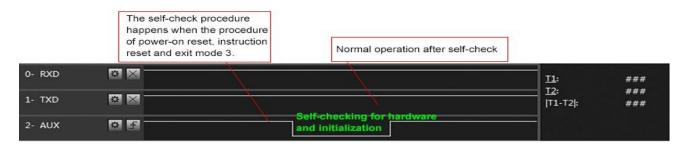
Timing Sequence Diagram of AUX when self-check
