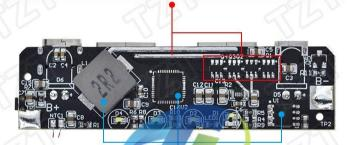
The main control chip and protection chip are not provided with reverse connection protection for this motherboard. Please do not put the battery upside down.
