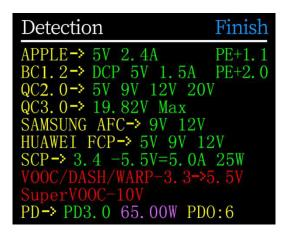
In this mode, The meter tries to trigger various protocols in turn, Display the test results on the screen, Red is not supported, Green is support, In the process of testing, Such as measuring PD chargers, It is normal to restart and continue testing. During the test, it is forbidden to connect to any equipment at the back end.
