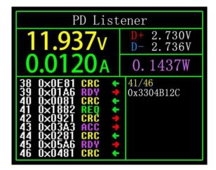
Click the middle button, Can switch to the page of "View detailed communication process", As shown above. Left column, You can select the message to be viewed by left/key, Such as:
