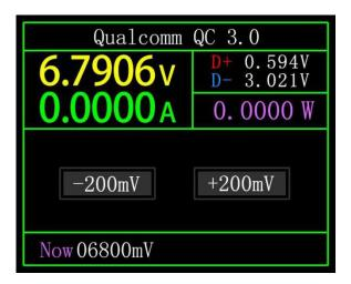
In QC3.0 trigger mode, Use the left and right keys to decrease/increase the trigger voltage, Click BACK to return. Press the left/right keys to quickly decrease/increase the voltage.
