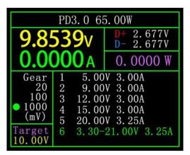
Switch the PD communication switch to ON, Enter the PD protocol trigger mode. After exiting the PD trigger, switch the PD communication switch to OFF.
