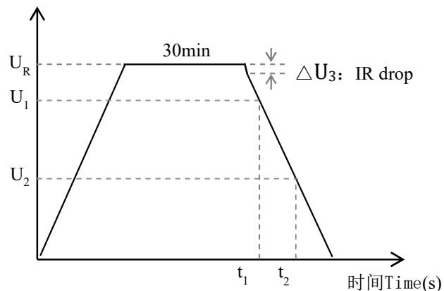
$$\text{容量计算方式} \quad \text{Capacitance calculation : } C = I \times \frac{t_2 - t_1}{U_1 - U_2}$$
