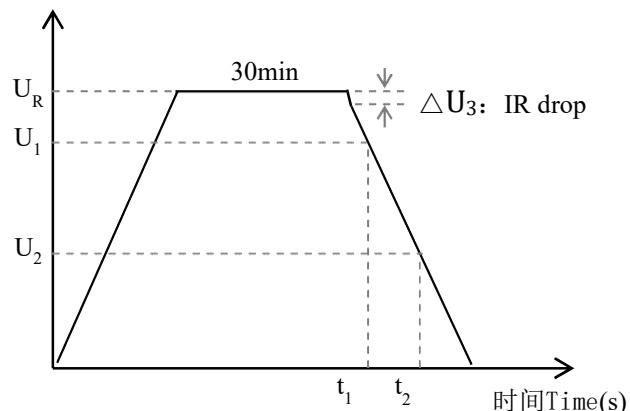
$$\text{容量计算方式} \quad \text{Capacitance calculation : } C = I \times \frac{t_2 - t_1}{U_1 - U_2}$$
