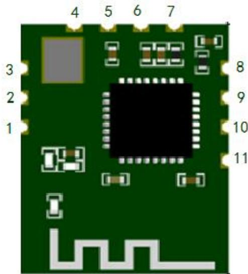
Fig. 2. Module Pins Distribution Diagram (Top View)
