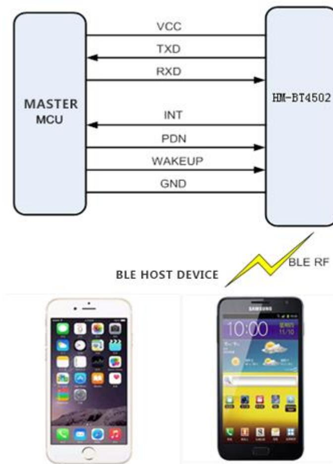
Figure 1. Application Schematic of the Pass-through Module
