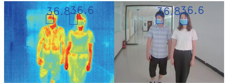
The blue temperature value and blue box indicate that the body temperature is normal.
