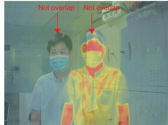
The image does not overlap. Unable to recognize human face and display the temperature.
