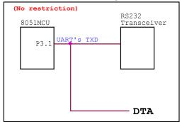
Figure 5: P3.1 is pulled low.
