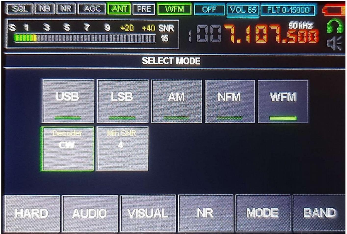
The MODE menu is used to select the type of modulation and to control decoders (Such as TTY/CW). You can exit by pressing the MODE button or by clicking on the ENC\_VOL encoder.
