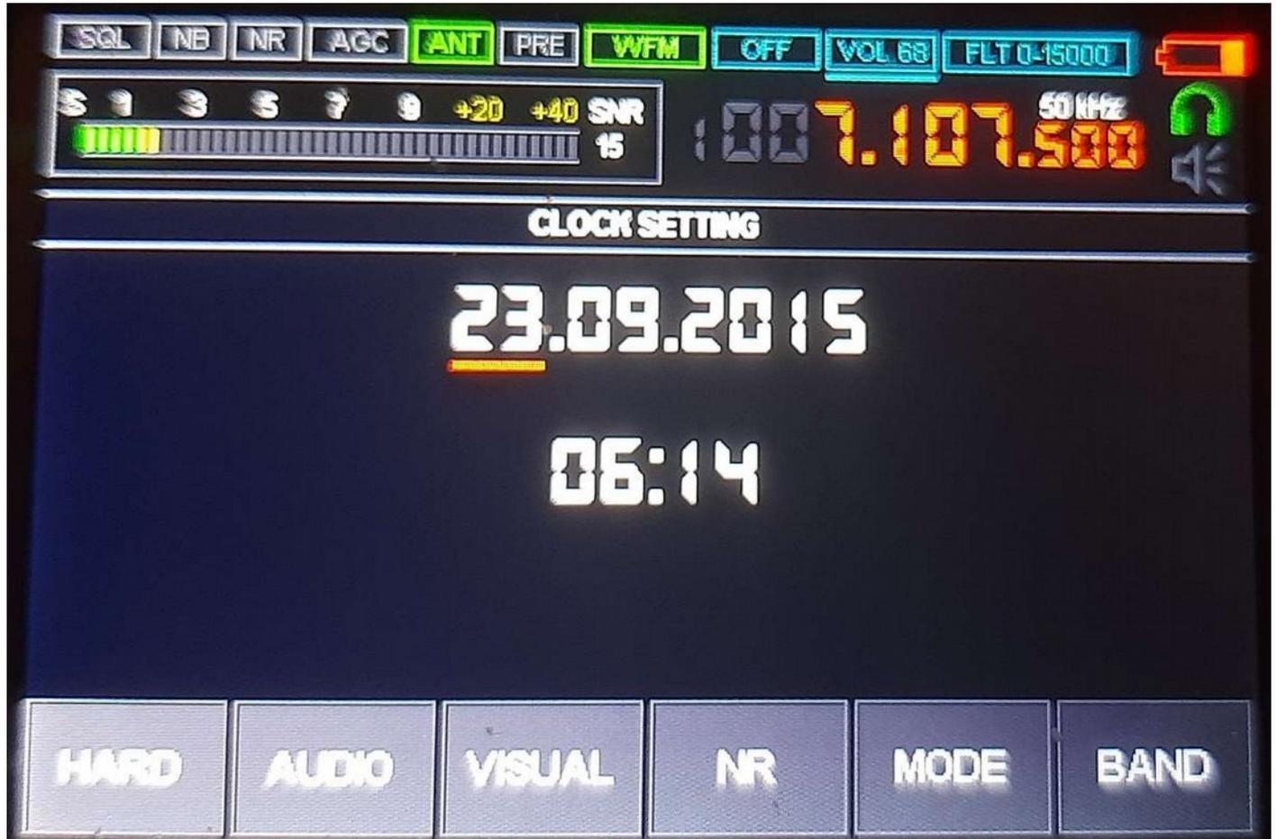
This page is designed for setting the clock. You can enter this menu by long pressing the HARD button. Setting is performed by using the ENC\_VOL and its button. To save, long press the ENC\_VOL button until there is a beep sound. Exit by pressing the HARD button. You can exit to the main screen of the receiver by clicking on the the ENC\_FREQ button. (The time will not be saved if you exit before saving.)
