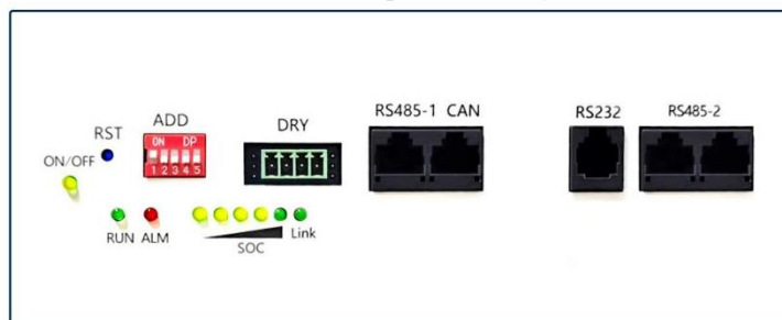
从机地址8设置示例(Example of Setting Slave Address 2)
