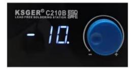
If the measured temperature is 10 °C lower than the actual temperature, the knob is turned clockwise and adjusted to 10.
