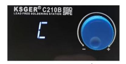
Press and hold the knob, then turn on the power, both into the Celsius and Fahrenheit conversion.
