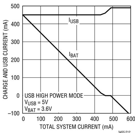
Figure 12. Charge Current vs Total System Current
