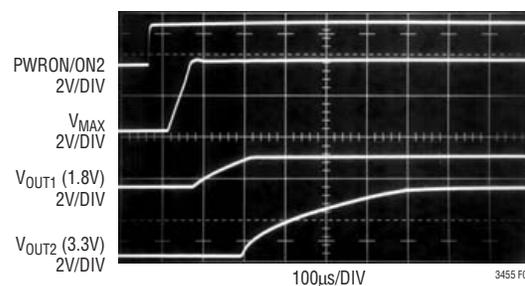
Figure 4. Sequencing for Switcher 1 and 2 Outputs
