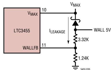
Figure 5. Schottky Leakage Current Path
