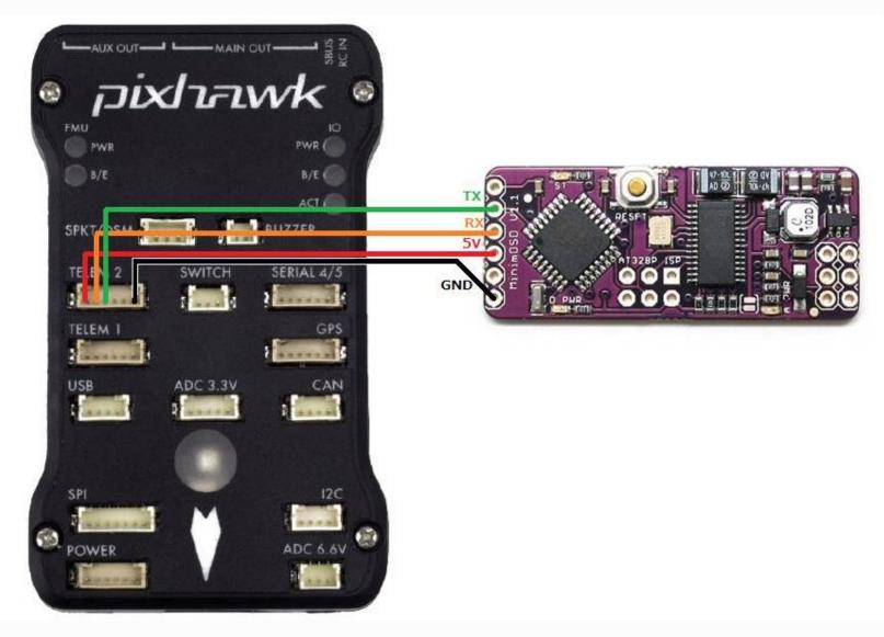
Set SERIALx\_PROTOCOL = 1 (MAVLink1) because MinimOSD does not understand MAVLink2 **Basic wiring Diagram**
