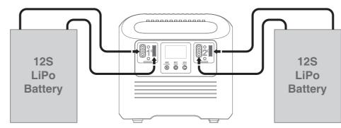
5) Select the Charge Mode: Fast Charge or Charge, and long-press the START button for three seconds to start charging.
