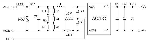
Figure 1. Circuit for EMC Enhancement
