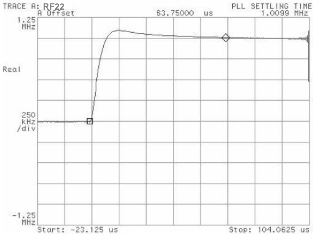
Figure 51. Synthesizer Settling Time for 1 MHz Jump Settled within 10 kHz
