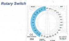
mA µA COM Turn off the product at this position. The product automatically powers off after 15 minutes of inactivity. The built-in beeper beeps 5 times 1 minute before auto power off. To restart the product from auto power off, press the HOLD button OFF or turn the rotary switch back to the OFF position and then to a needed position. To disable the Auto Power Off function, hold down the SELECT button when turning on the product, you will hear five beeps if
