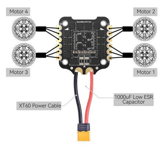
■ Note: In order to prevent the stack from being burnt out by voltage spikes on powering up, it is strongly recommended to use the Low ESR capacitor in the package.
