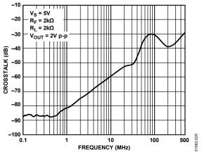
Figure 25. AD8052 Crosstalk (Output-to-Output) vs. Frequency
