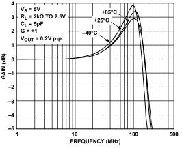
Figure 12. AD8054 Gain vs. Frequency vs. Temperature
