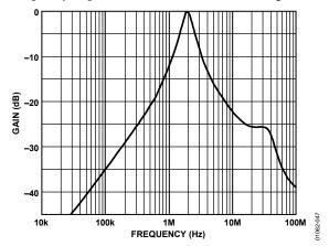
Figure 47. Frequency Response of 2 MHz Band-Pass Biquad Filter
