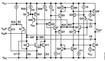
Figure 40. AD8051/AD8052 Simplified Schematic
