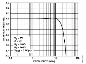
Figure 13. AD8051/AD8052 0.1 dB Gain Flatness vs. Frequency; G = +2
