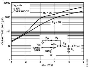
Figure 44. AD8051/AD8052 Capacitive Load Drive vs. Closed-Loop Gain
