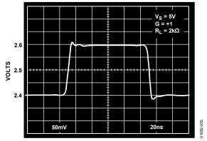
Figure 35. AD8051/AD8052 200 mV Step Response;  $V_S = 5 \text{ V}$ , G = +1
