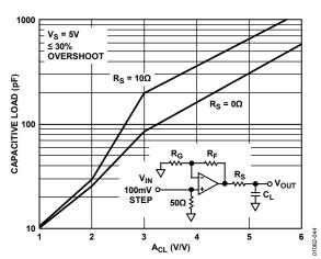
Figure 45. AD8054 Capacitive Load Drive vs. Closed-Loop Gain
