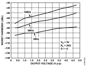
Figure 20. Worst Harmonic vs. Output Voltage
