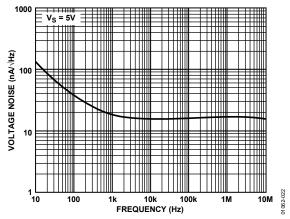
Figure 22. Input Voltage Noise vs. Frequency
