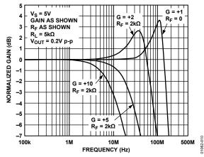
Figure 10. AD8054 Normalized Gain vs. Frequency;  $V_S = 5 V$
