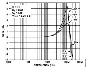
Figure 11. AD8054 Gain vs. Frequency vs. Supply
