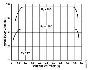
Figure 32. Open-Loop Gain vs. Output Voltage
