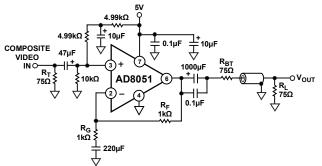
Figure 52. Single-Supply Composite Video Line Driver
