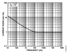
Figure 23. Input Current Noise vs. Frequency
