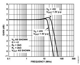
Figure 17. AD8054 Large Signal Frequency Response; G = +2
