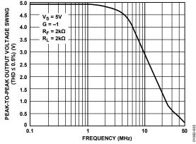
Figure 5. Low Distortion Rail-to-Rail Output Swing
