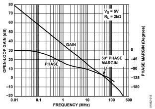
Figure 15. AD8051/AD8052 Open-Loop Gain and Phase vs. Frequency
