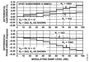
Figure 21. AD8051/AD8052 Differential Gain and Phase Errors
