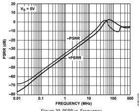
Figure 29. PSRR vs. Frequency
