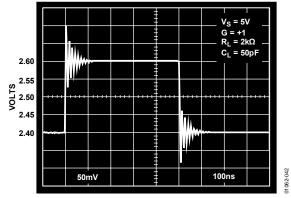
Figure 43. AD8051/AD8052 200 mV Step Response;  $C_L = 50 \text{ pF}$
