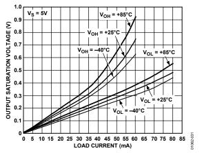
Figure 31. AD8051/AD8052 Output Saturation Voltage vs. Load Current
