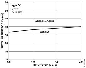
Figure 30. Settling Time vs. Input Step
