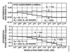
Figure 24. AD8054 Differential Gain and Phase Errors
