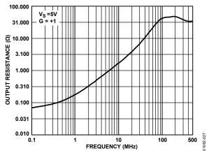
Figure 27. Closed-Loop Output Resistance vs. Frequency
