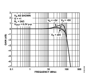
Figure 8. AD8051/AD8052 Gain vs. Frequency vs. Supply
