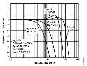
Figure 7. AD8051/AD8052 Normalized Gain vs. Frequency;  $V_S = 5 V$
