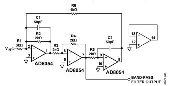
Figure 46. 2 MHz Biquad Band-Pass Filter Using AD8054
