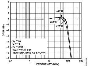
Figure 9. AD8051/AD8052 Gain vs. Frequency vs. Temperature
