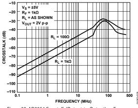
Figure 28. AD8054 Crosstalk (Output-to-Output) vs. Frequency
