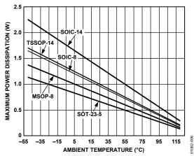
Figure 6. Maximum Power Dissipation vs. Temperature for AD8051/AD8052/AD8054
