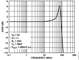
Figure 42. AD8051/AD8052 Closed-Loop Frequency Response;  $C_L = 50 \text{ pF}$
