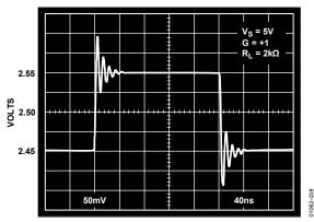
Figure 38. AD8054 100 mV Step Response;  $V_S = 5 V$ , G = +1
