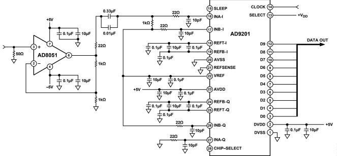
Figure 50. The AD8051 Driving an AD9201, a 10-Bit, 20 MSPS Analog-to-Digital Converter Rev. H | Page 19 of 24
