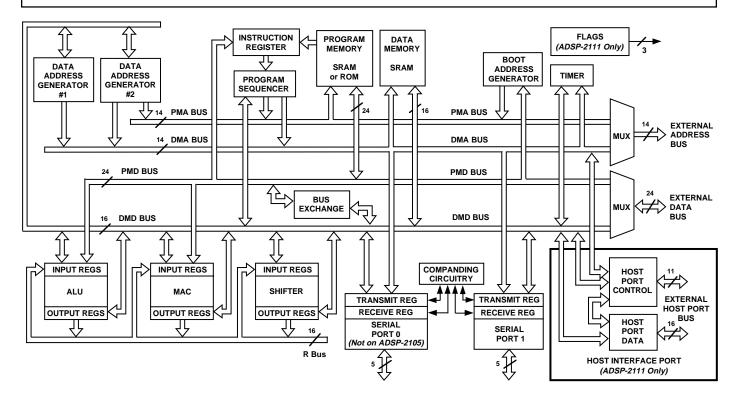
Figure 1. ADSP-21xx Block Diagram
