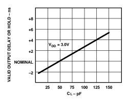
Figure 25. Typical Output Valid Delay or Hold vs. Load Capacitance, C<sub>1</sub> (at Maximum Ambient Operating Temperature)
