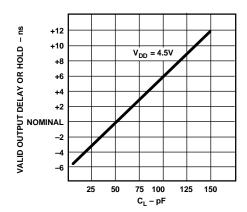
Figure 19. Typical Output Valid Delay or Hold vs. Load Capacitance, C<sub>L</sub> (at Maximum Ambient Operating Temperature)
