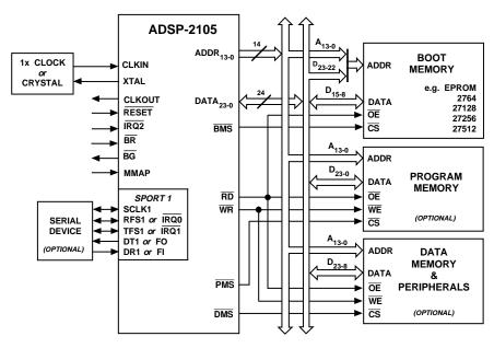
THE TWO MSBs OF THE DATA BUS (D $_{23-22}$ ) ARE USED TO SUPPLY THE TWO MSBs OF THE BOOT MEMORY EPROM ADDRESS. THIS IS ONLY REQUIRED FOR THE 27256 AND 27512.
