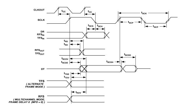
Figure 34. Serial Ports
