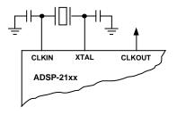
Figure 2. External Crystal Connections
