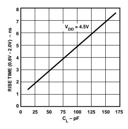
Figure 12. Typical Output Rise Time vs. Load Capacitance, C<sub>1</sub> (at Maximum Ambient Operating Temperature)
