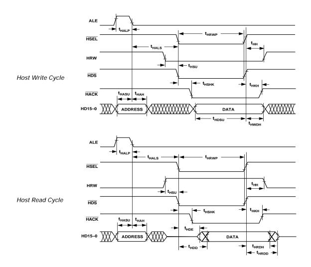
Figure 38. Host Interface Port (HMD1 = 1, HMD0 = 1)
