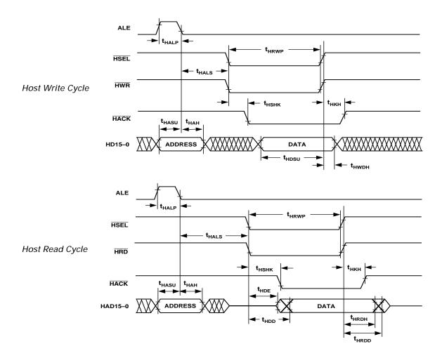
Figure 37. Host Interface Port (HMD1 = 1, HMD0 = 0)
