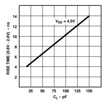
Figure 18. Typical Output Rise Time vs. Load Capacitance, C<sub>1</sub> (at Maximum Ambient Operating Temperature)
