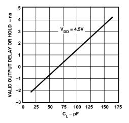
Figure 13. Typical Output Valid Delay or Hold vs. Load Capacitance, C<sub>L</sub> (at Maximum Ambient Operating Temperature)
