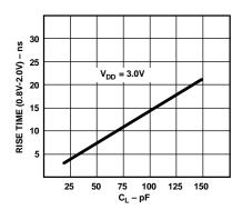
Figure 24. Typical Output Rise Time vs. Load Capacitance, C. (at Maximum Ambient Operating Temperature)
