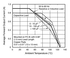
Fig. 1 - Derating Curves Output Rectified Current for B40C800D...B125C800DM
