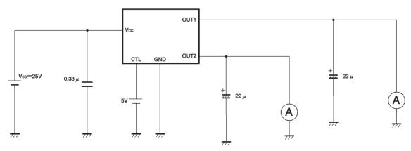
Fig.5 Circuit for measuring output short-circuit current
