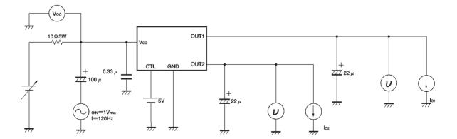
Vcc = 13 V,  $I_{01} = 500 mA$  when measuring the ripple rejection ratio 1 Vcc = 13 V,  $I_{02} = 350 mA$  when measuring the ripple rejection ratio 2
