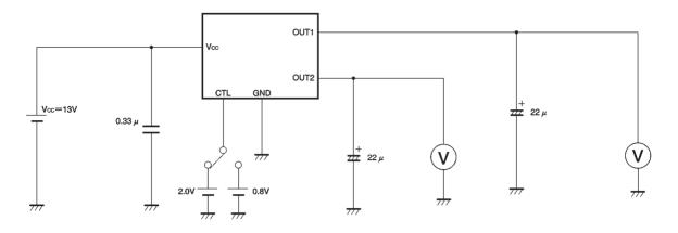
Fig.6 Circuit for measuring mode switching voltage
