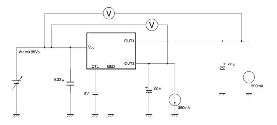
Fig.3 Circuit for measuring minimum I/O voltage differential
