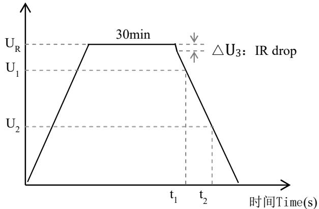
容量计算方式 Capacitance calculation:  $C = I \times \frac{t_2 - t_1}{U_1 - U_2}$
