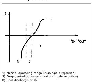
Figure 4 : Supply voltage Rejection vs. Input Voltage.
