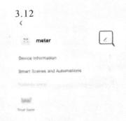
If device connect successfully, you can realize remote control on/off, timer control and delay time control, and read the energy /current/ voltage/active power and history energy. you also can change the device name and share the device to others.
