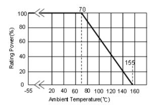
Fig.1 Power Derating Characteristics
