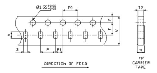
Remark : Pitch tolerance over any 10 pitches of Po is  $\pm\,0.2~\text{mm}$
