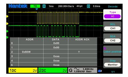
ADDR: In the address bar, "R" represents the read operation, and "W" represents the write operation;
