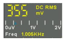
The display in the middle of the DVM box is the corresponding ratio of the current measured voltage value to the range corresponding to the eight vertical grids on the screen with the selected volt/div (turn the volt/div knob).
