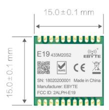
Since the module is a pure RF transceiver module, you need to use the MCU driver or a dedicated SPI debug tool.
