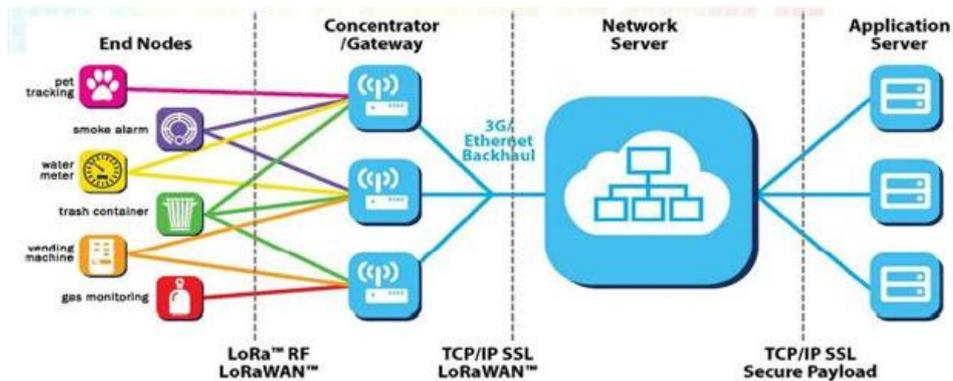
The complete LoraWan network system consists of: node, gateway, Lora NetWork Server, application server, the node is generally designed by LORA chip; the gateway is designed by SX1301 provided by semtech; Lora NetWork Server now has open source lorasever or commercial TTN (The ThingsNetwork), users can build their own; application server is designed and developed by users, mainly used for data exchange with Lora NetWork Server applications.
