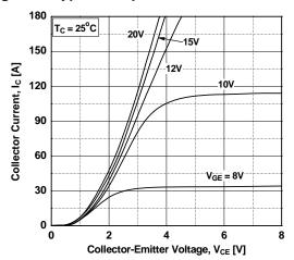
**Figure 2. Typical Output Characteristics**
