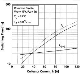
Figure 16. Turn-off Characteristics vs.
