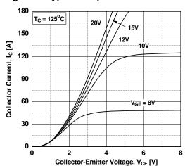
Figure 3. Typical Saturation Voltage Characteristics
