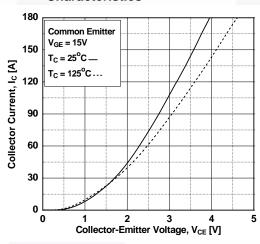
Figure 4. Transfer Characteristics
