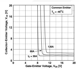
Figure 7. Saturation Voltage vs. V<sub>GE</sub>
