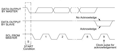
Figure 5. Acknowledge on the I<sup>2</sup>C Bus
