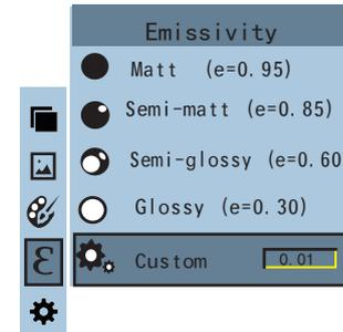
As shown in the figure, press “**MENU**” key to enter the main menu and select “**ε**”(emissivity) option and press “**▶**” key to enter the emissivity list.
