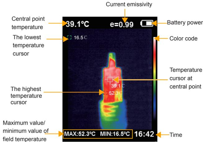
1. Color code: used to mark the color corresponding to the relative temperature from low to high in the field of version.
