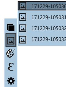
As shown in the figure, Then press “**IR**” key to enter image list. Press “**UP**” or “**DOWN**” key in navigation to select the image. Then press “**SELECT**” key to view image. When viewing the images, press “**IR**” key to view the precious image, Press “**IR**” to view the next image. Press “**ENTER**” key to return. Press “**MENU**” key to exit from the menu.
