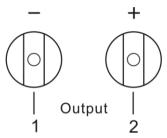
! When output current greater than 20A, connect negative wires with "1" terminals, and positive wires with "2" terminals.
