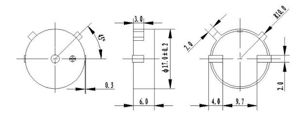
Rated Voltage: 12Vp-pOperating Voltage:  $1\sim30Vp-p$ Max.Rated Current: 12mA
