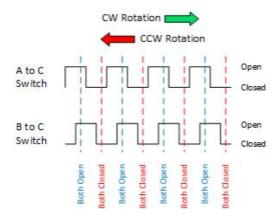
Essentially, determining which switch changed states first is how the direction of rotation is determined. If A changed states first, the switch is rotating in a clockwise direction. If B changed states first, the switch is rotating in a counter clockwise direction.
