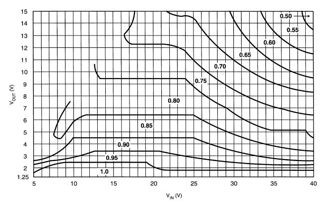
Figure 23. LM2825 Output Current Derating for  $T_A = 70^{\circ}C$  to 85°C
