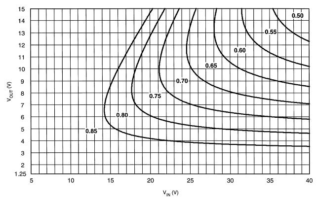
Figure 20. LM2825 Output Current Derating for  $T_J = -40^{\circ}C$  to  $-25^{\circ}C$
