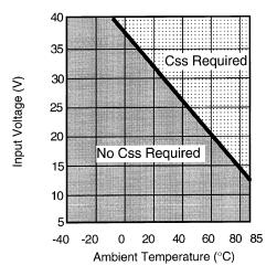
Figure 19. Usage of the Soft-start Capacitor
