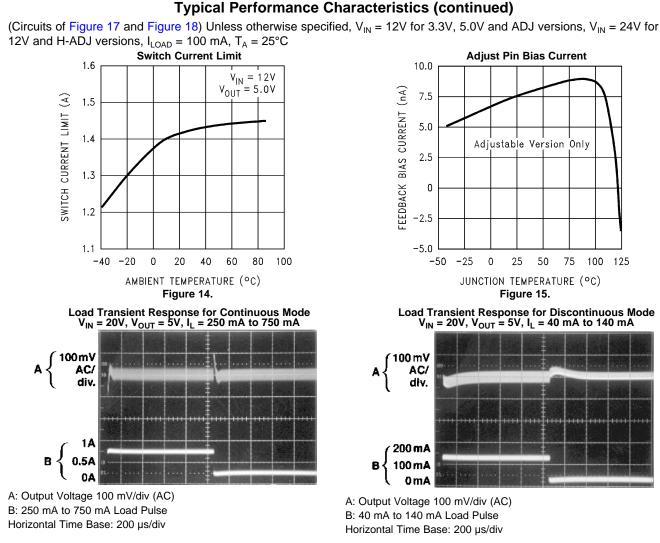
Figure 16. Typical Load Transient Response
