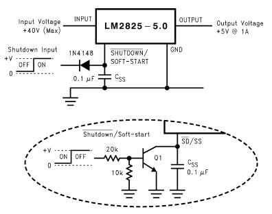
Figure 24. Typical Circuits Using Shutdown/Soft-start Features
