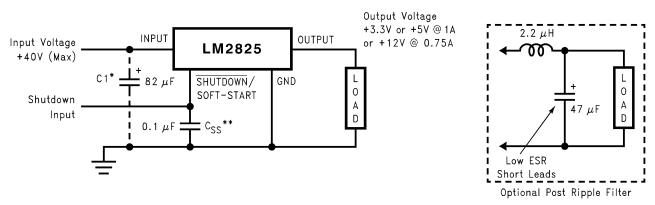
\*Optional—Required if package is more than 6" away from main filter or bypass capacitor. \*\*Optional Soft-start Capacitor
