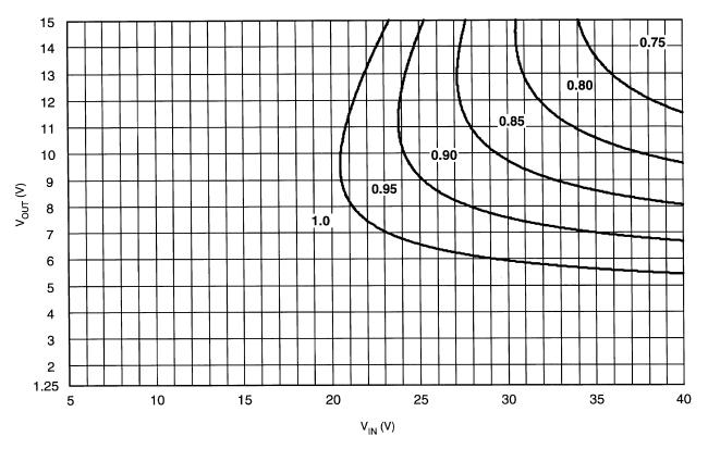
Figure 22. LM2825 Output Current Derating for  $T_A = 0^{\circ}C$  to 70°C
