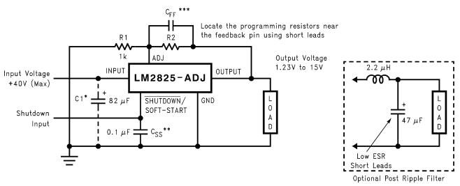
\*Optional—Required if package is more than 6" away from main filter or bypass capacitor.
