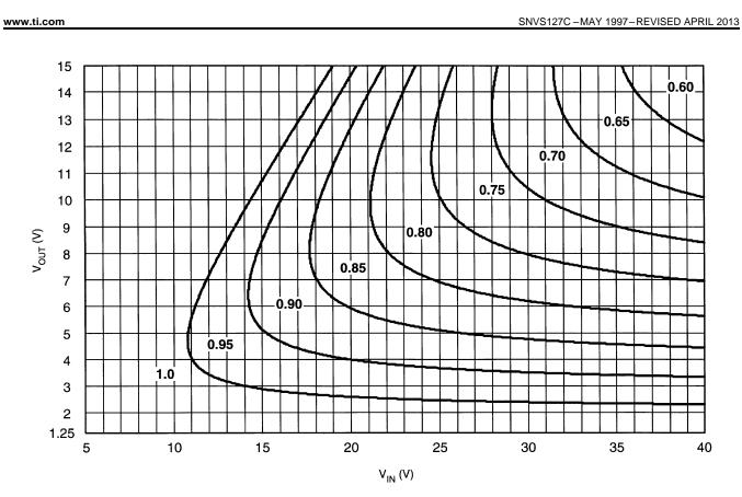
Figure 21. LM2825 Output Current Derating for  $T_J = -25^{\circ}C$  to  $0^{\circ}C$
