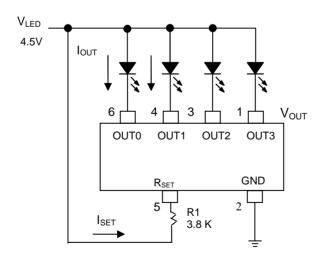
Neither a capacitor, an inductor nor Schottky diode is needed.
