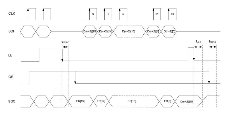
1. Conditions required to activate the open-circuit detection: (1) falling edge of LE and (2)  $\overline{OE}$  =High
