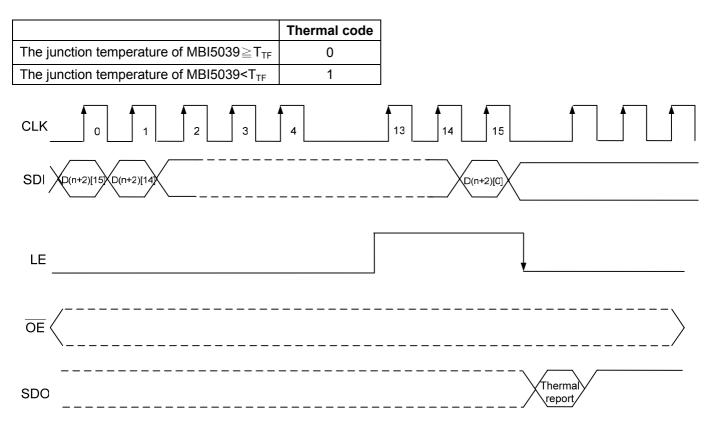
At the falling edge of LE, if the driver is overheated, the code "7FFF(HEX)" is delivered to SDO; otherwise, the code "FFFF(HEX)" is latched to sift register.
