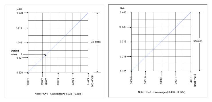
The 6 bits (bit 5~bit 0) of the configuration register set the gain of output current, i.e., G. As total 6-bit in number, i.e., ranged from 6'b000000 to 6'b111111, these bits allow the user to set the output current gain up to 64 levels. These bits can be further defined inside configuration register as follows:
