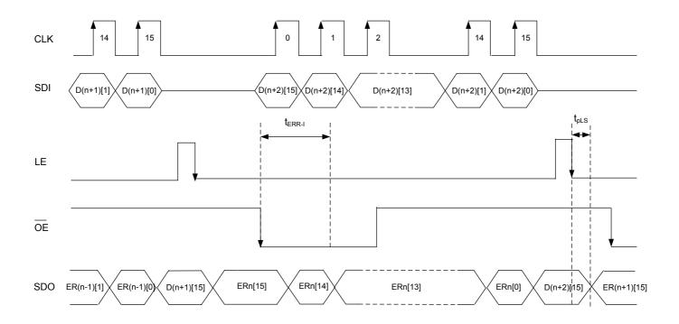
1. Condition of valid error detection: (1) Data ="1" (2)  $\overline{OE}$  (low) > t<sub>ERR-I</sub>
