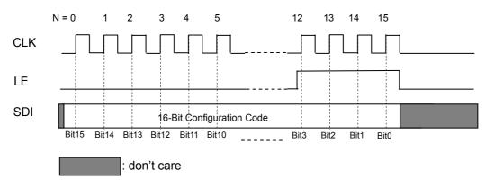
After entering the writing configuration mode, the system controller sends a 16-bit configuration register to 16-bit shift register through the SDI pin. Then the falling edge of LE will transfer the contents in the shift register to a 16-bit configuration register rather than the 16-bit output latch.
