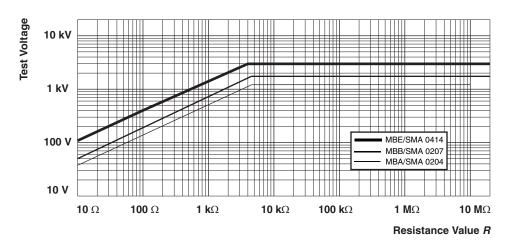
Pulse load rating in accordance with IEC 60115-1, 4.27; 10  $\mu$ s/700  $\mu$ s; 10 pulses at 1 minute intervals; 10/700 Pulse for permissible resistance change 0.5 %.
