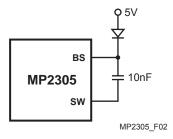
Figure 2—External Bootstrap Diode
