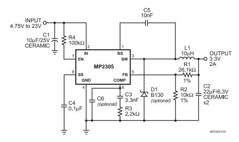
Figure 3—MP2305 with 3.3V Output, 22µF/6.3V Ceramic Output Capacitor
