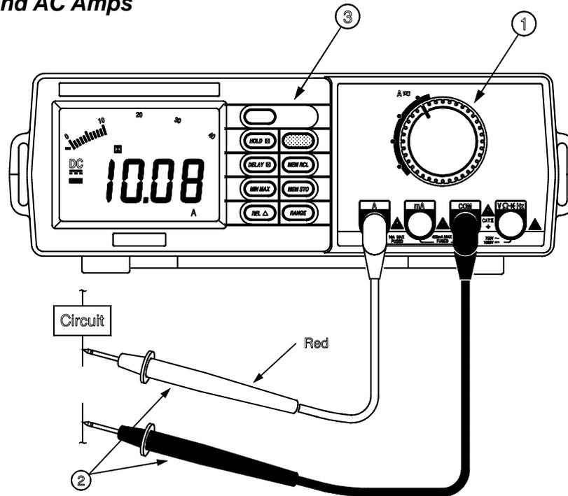
**Figure 2-3. Amps Measurements**
