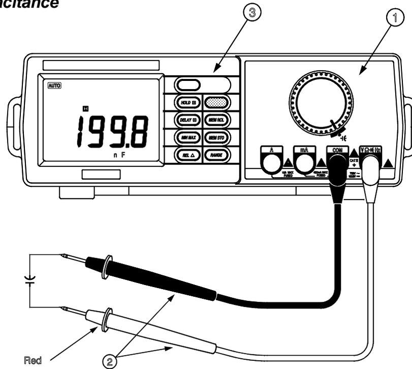
**Figure 2-6. Capacitance Measurements**
