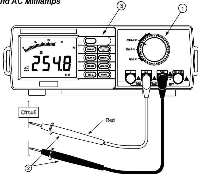
**Figure 2-4. Milliamps Measurements**
