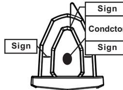
\* When measuring AC current, place the conductor to be measured in the center position of clamp head. If it is not in the center position, it can increase error by 1.5%
